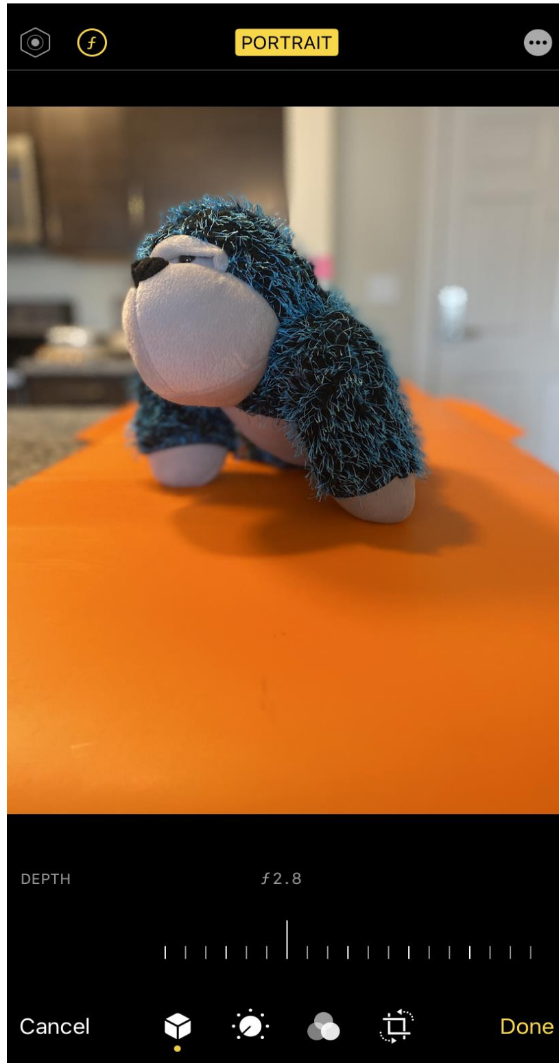
Fig. 19 iPhone Screenshot of Editing Mode for Photo Captured Using Portrait Mode with Blurred Background. Select the f icon in top left to access DEPTH slider and adjust the slider from f2.8 (default) to maximum f value ( f16 ) to remove background blur.
