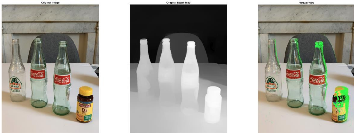
Fig. 3 Original Left View, Original Depth Map, and Virtual Right View with No Hole-Filling
