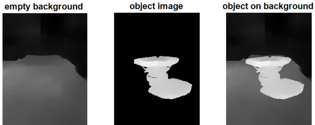
Fig. 17 Empty Environment Depth Map (left), Extracted Object Depth Map (center), Superimposed Object Depth Map (right)
