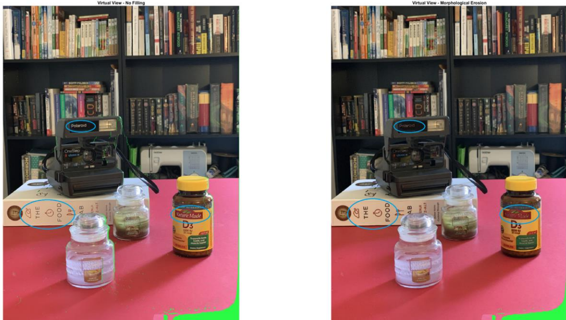
Fig. 8 Virtual View without Hole-Filling (left) and Virtual View Processed by Morphological Erosion (right)
