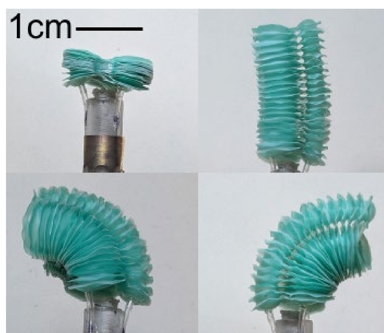
Stacked balloon actuator in various configurations.
