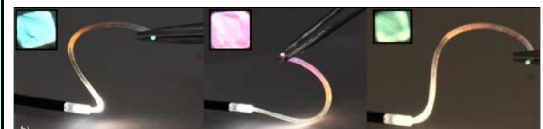
Figure 3: Close-up of shape sensing core tip (what RGB sensor detects)
