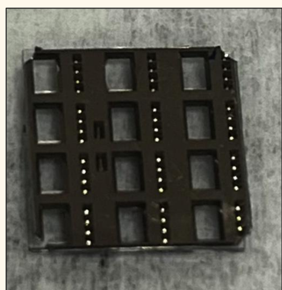
Figure 3. The Si chip. The large rectangles are the reservoirs, and the small rectangles are the membranes that the nanopores are drilled into.
