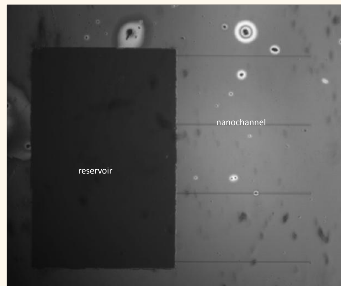
Figure 6. The channel drains and the meniscus recedes from left (top) to right (bottom) as the water evaporates.
