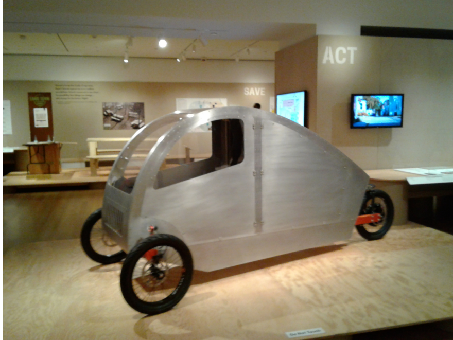
"Orbit," a fully electric, enclosed vehicle from the "Future Cycles" series by Cameron and Rachael Van Dyke ("The Future People"), Michigan, 2012-present. Aluminum, steel, electric motor and controller, battery, bicycle parts. Photo courtesy of the author.
