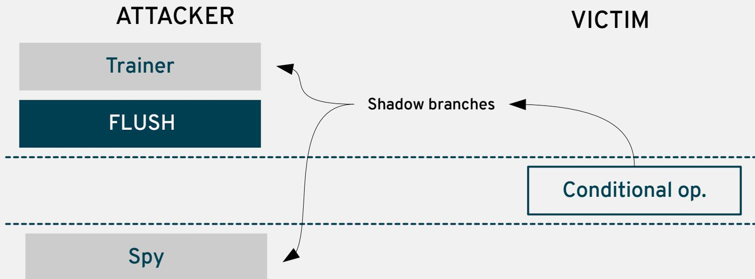
Train the branch predictor then flush your own caches for the “spy” branch. Let the victim code run, then run your own “spy” branch. See if the “trainer offset” flushed line was loaded by the “spy” (measure time to access). If not, the victim branch fired and retrained the BP.
