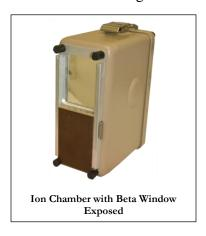
therefore cannot be detected, but the overall accumulation of charge in the air can be measured. Higher-energy particles create more ion pairs, so the signal is proportional to exposure rate, which is proportional to dose rate.
