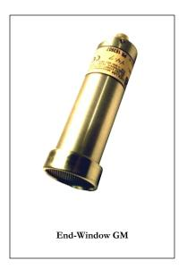
gammas (e.g. I-125) or low-energy betas (e.g. H-3) cannot be detected by a Geiger counter, so other instruments must be used.
