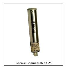
laboratory setting, as a significant amount of activity must be present to give a reliable reading. This detector is common in clinical areas where exposure rate is a concern, although a regular GM or NaI detector should still be used to locate contamination. Some energy-compensated detectors are completely contained inside a ratemeter to prevent damage and increase ease of use.
