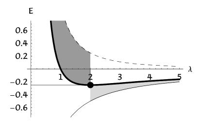
Qualitative dependence of hydrogen atom potential energy (thin curve), kinetic energy (dashed curve), and total energy (thick curve) versus wavelength of the electron matter wave. The attractive force due to potential energy dominates when the atom is large, that is, at larger matter wave wavelengths (light shaded region), while repulsive force due to kinetic energy dominates when the atom is small, that is, at smaller matter wave wavelengths (dark shaded region).
