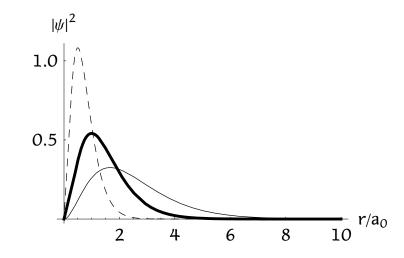
Cross section through alternative hydrogen atom lowest energy spatial distributions,  $|\psi|^2$ . Distance from the nucleus, *r*, is in units  $a_0 = 0.529$  Å. The thick line is for the correct spherical wave; the thin line is for a spherical wave that is too diffuse; and the dashed line is for a spherical wave that is too compact.
