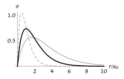
Cross section through alternative hydrogen atom lowest energy spherical waves,  $\psi$ . Distance from the nucleus, r, is in units  $a_0 = 0.529$  Å. The thick line is the correct spherical wave; the thin line is a spherical wave that is too diffuse; and the dashed line is a spherical wave that is too compact.
