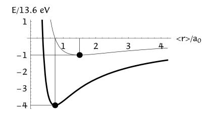
Hydrogen atom (thin line) and helium ion (thick line) average total energy (thick curve) versus average size  $\langle r \rangle$  of the spherical wave of the lowest energy state. Energy is in units of the ionization energy of hydrogen atom, 13.6 eV, and size in units of the Bohr radius,  $a_0 = 0.529$  Å.
