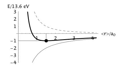
Hydrogen atom average potential energy (thin curve), average kinetic energy (dashed curve), and average total energy (thick curve) versus average size  $\langle r \rangle$  of the spherical wave of the lowest energy state of the atom. Energy is in units of the ionization energy of hydrogen atom, 13.6 eV, and size in units of the Bohr radius,  $a_0 = 0.529$  Å. The energy minimum at  $\langle r \rangle = 1.5$ , E = -1 is the observed value for hydrogen atom.
