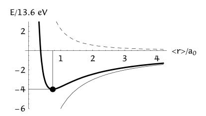
Helium ion average potential energy (thin curve), average kinetic energy (dashed curve), and average total energy (thick curve) versus average size  $\langle r \rangle$  of the spherical wave of the lowest energy state of the ion. Energy is in units of the ionization energy of hydrogen atom, 13.6 eV, and size in units of the Bohr radius,  $a_0 = 0.529$  Å. The energy minimum at  $\langle r \rangle = 0/75$ , E = -4 is the observed value for helium ion.
