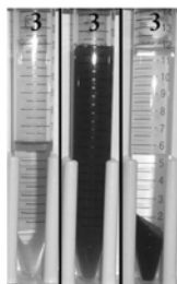
Mixture 3 is shown before and after addition of phosphate and after centrifugation.
