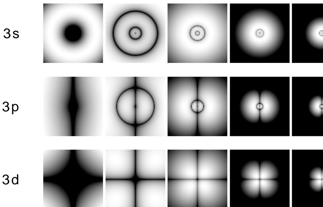
Hydrogen atom  $n = \text{radial loops} + \text{nodal planes} = 3$  family: 3s, 3p, and 3d, energy  $-13.6 \text{ eV} / 3^2 = -1.51 \text{ eV}$ . Probability density in the  $xy$  plane. The nucleus is at the center. From left to right, the width and height are 0.1, 1, 3, 6, and 9 nm. The brightness of the display is proportional to the probability density.
