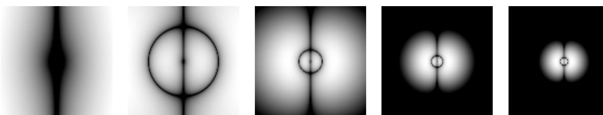
Probability density in the  $xy$  plane of the  $3p_x$  hydrogen atom electron wave (wave function). The nucleus is at the center. From left to right, the width and height are 0.1, 1, 3, 6, and 9 nm. The brightness of the display is proportional to the probability density.
