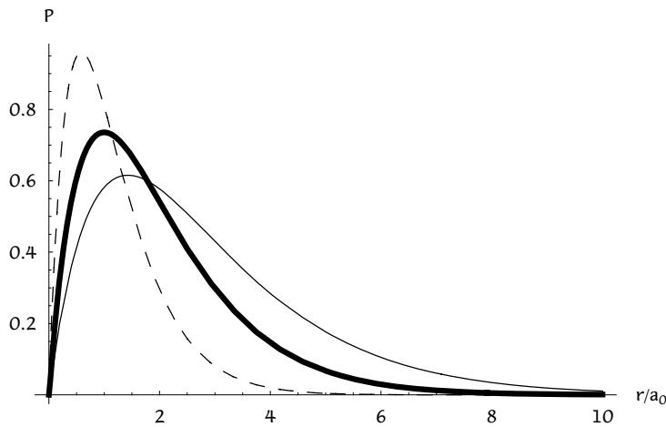
Lowest energy s ( $\ell = 0$ ) shell amplitudes for hydrogen atom. Distance from the nucleus,  $r$ , is in units  $a_0 = 0.529 \text{ \AA}$ . The thick line is the correct shell amplitude and its energy -1; the thin line is a shell amplitude that is too diffuse; and the dashed line is a shell amplitude that is too compact.
