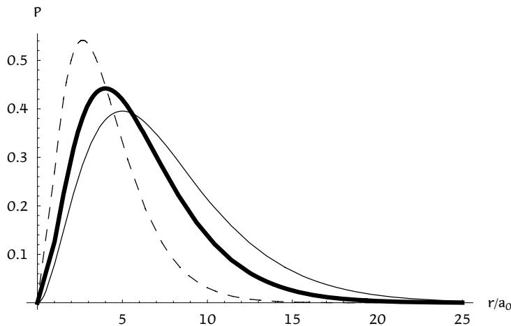
Lowest energy p ( $\ell = 1$ ) shell amplitude for hydrogen atom. Distance from the nucleus,  $r$ , is in units  $a_0 = 0.529 \text{ \AA}$ . The thick line is the correct shell amplitude and its energy is -1/4; the thin line is a shell amplitude that is too diffuse; and the dashed line is a shell amplitude that is too compact.
