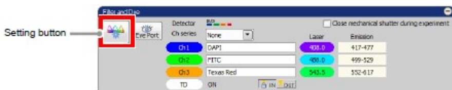
Figure 5.3-2 Filter and Dye window
