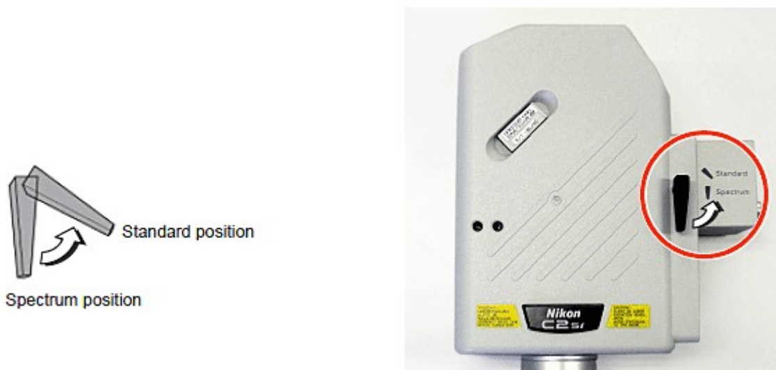
Figure 5.3-23 Switching the optical path of the C2 scan head
