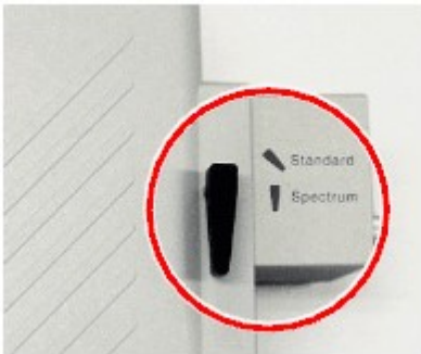
Figure 16.1-1 Optical path changeover lever for C2 scan head
