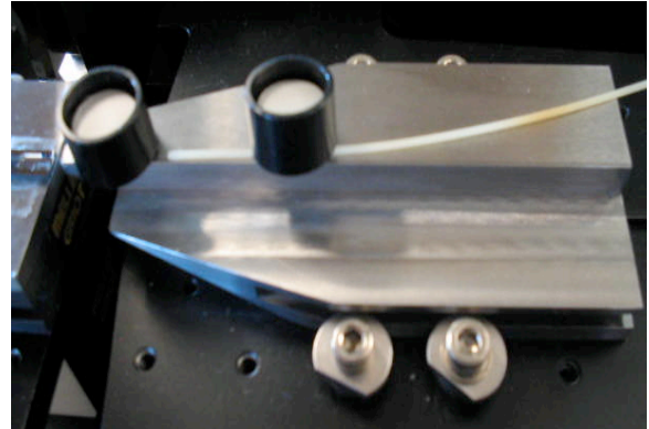
Fig. 1: On the left: The throughput of the microring resonators measured with the fiber array assembly. Q ( \sim 11,500 ) is as high as expected, however the throughput is still around -25dB. On the right: The fiber holder for array assembly to increase the throughput. The fiber to be placed is put in the groove on the fiber holder and placed in one of the v-grooves in the array. The holder is milled down on one side to allow for placing the second fiber without damaging the assembly of the first one.
