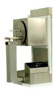
✓ The use of twin alumina rods provides a cost effective, readily available material in lieu of long lead and expensive SIC type paddles. It also allows for the flexibility to change the inexpensive quartz sheaths for multi use furnace tubes in lieu of cleaning SIC.
