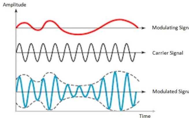
*In VLC signals, optical intensity is modulated. Carrier frequency is NOT required. Technically, the signal is modulated in THz*
