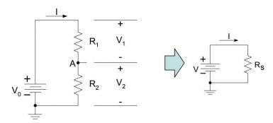
$$V_0 = V_1 + V_2 = IR_1 + IR_2$$
