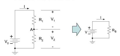
$$V_{0} = V_{1} + V_{2} = IR_{1} + IR_{2}$$
