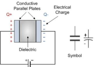
NOTE: Directly connecting a capacitor to a voltage supply is not practical.
