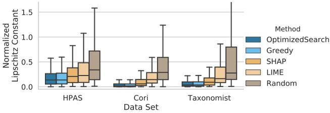
Fig. 6. Robustness of explanations to changes in the test sample. The *counterfactual time series explanation method* (OptimizedSearch and Greedy) is the most robust to small changes in the input, resulting in more predictable explanations and better user experience. Lipschitz constant is normalized to enable comparisons among data sets, and a lower value indicates better robustness.
