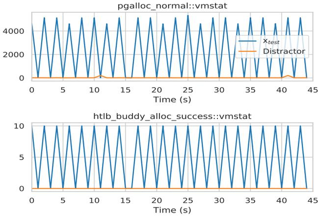
Fig. 2. The explanation of the *counterfactual time series explanation method* for correctly classified time window with the “memleak” label. The method provides two metrics as an explanation to change classification label from “memleak” to “healthy.” The metrics are shown in the  $y$ -axes and the metric names are above the plots.
