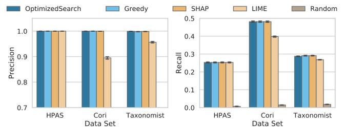
Fig. 5. Precision and recall of the explanations for a classifier with known feature importances. The *counterfactual time series explanation method* (OptimizedSearch and Greedy), and SHAP have perfect precision. LIME has lower precision for Cori and Taxonomist data sets, which indicates that although some features have no impact on the classifier decision, they are included in the LIME explanations. The low recall indicates that not every feature is used in every local decision.
