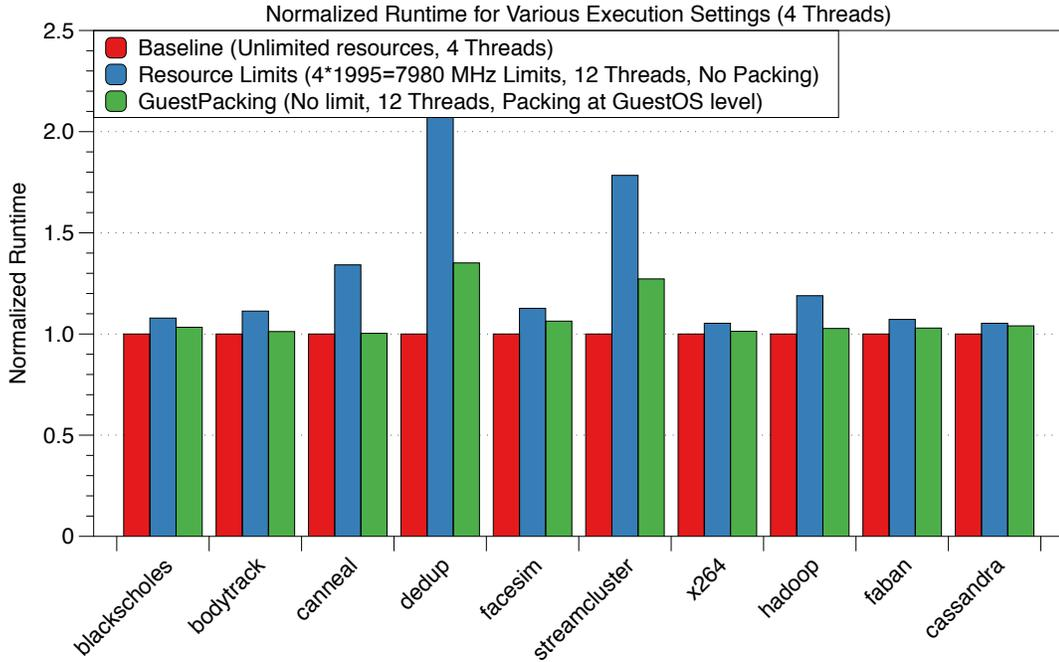
**Figure 5-6:** Performance overhead for running higher number of threads under power caps. Running applications with 12 threads and applying resource limits introduces large overheads for some of the applications. Packing the threads onto smaller number of vCPUs reduces the overhead up to 45%.
