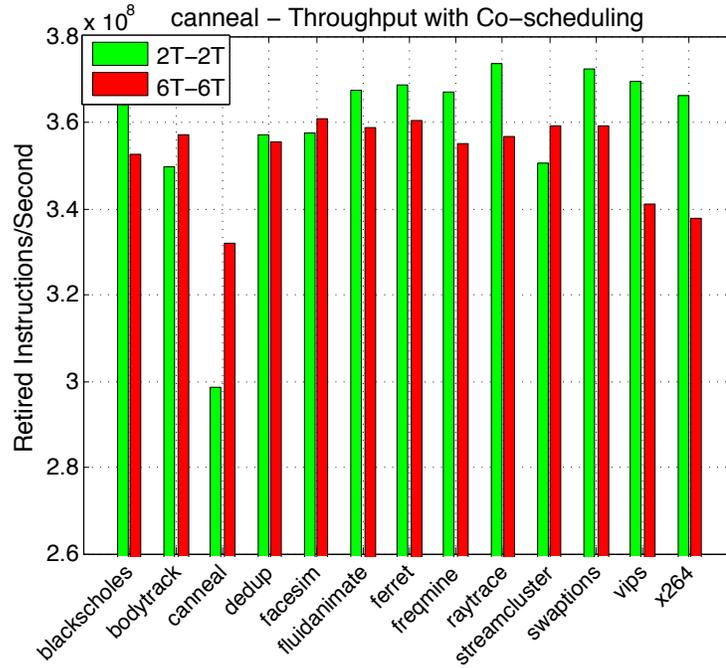
**Figure 4-7:** Performance comparison when `canneal` is co-scheduled with the other PARSEC benchmarks shown on the x axis. Figure demonstrates `canneal`'s throughput (per core) when each of the two co-scheduled applications runs with 2 threads and when each has 6 threads. Performance impact of co-scheduling is higher at 2 threads due to higher resource contention at the shared caches.
