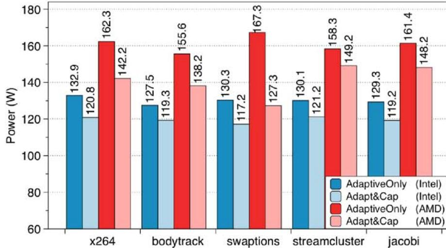
**Figure 5-22:** Comparison of power consumption for Adapt & Cap and only adaptive application under dynamically changing performance constraints. Adapt & Cap reduces the power consumption up to 27% compared to only application-level adaptation.
