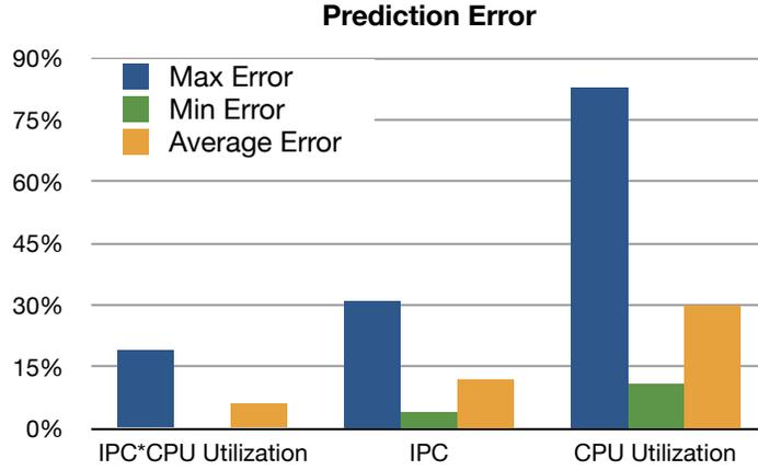
**Figure 4-11:** Maximum, minimum and average errors for predicting energy efficiency of PARSEC benchmarks for candidate metrics.
