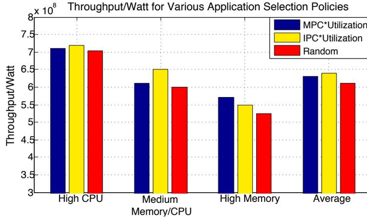
**Figure 4-8:** Throughput-per-watt for various benchmark sets that are co-scheduled with various policies. On average, randomly co-scheduling applications provides comparable energy efficiency in comparison to previously proposed based policies.
