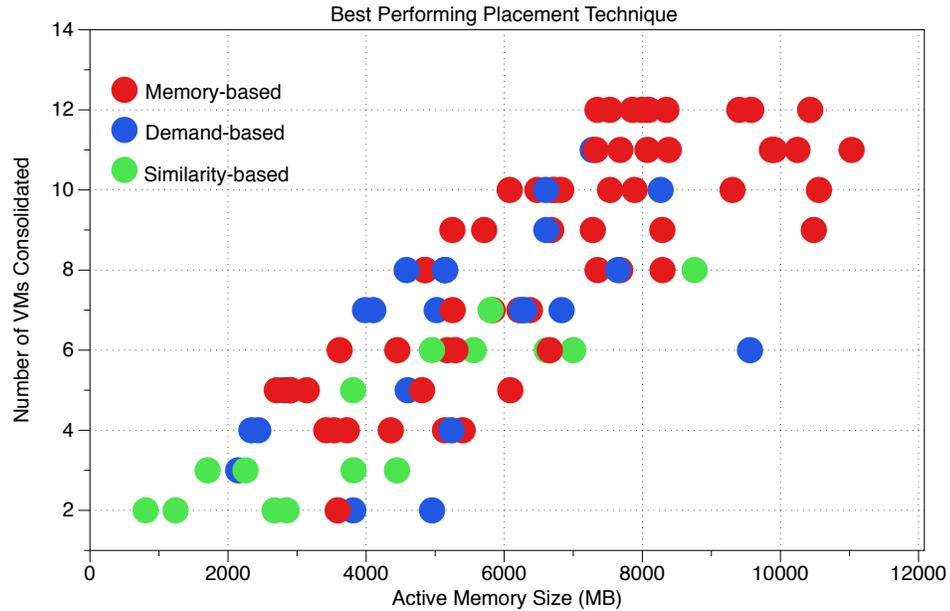
**Figure 5-17:** Best performing placement technique for various VM-density and active memory size. Memory-based technique is superior to other techniques with increasing number of VMs consolidated at the same time, which also leads to higher active memory size.
