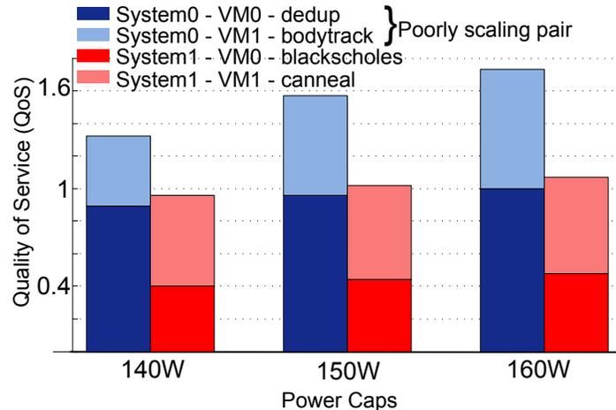
**Figure 5-3:** Overall normalized QoS of two distinct co-scheduling cases under various power caps. QoS range for the *scaling VMs* is much smaller than the *non-scaling VMs*. Thus, selecting non-scaling VMs to co-schedule have high potential for energy efficiency improvement.
