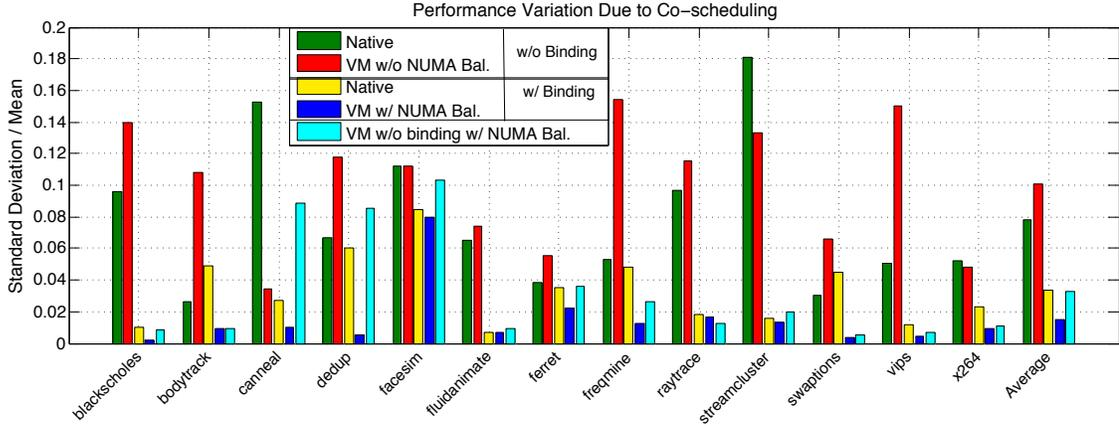
**Figure 4-9:** In this experiment, a PARSEC benchmark is co-scheduled with another benchmark (only two benchmarks at a time) under various CPU binding and NUMA balancing settings. The experiment is repeated to cover all possible application pairings. Figure shows the performance variation (standard deviation/mean) of each benchmark across its co-scheduled runs with the other benchmarks. Smaller bars indicate better performance isolation.
