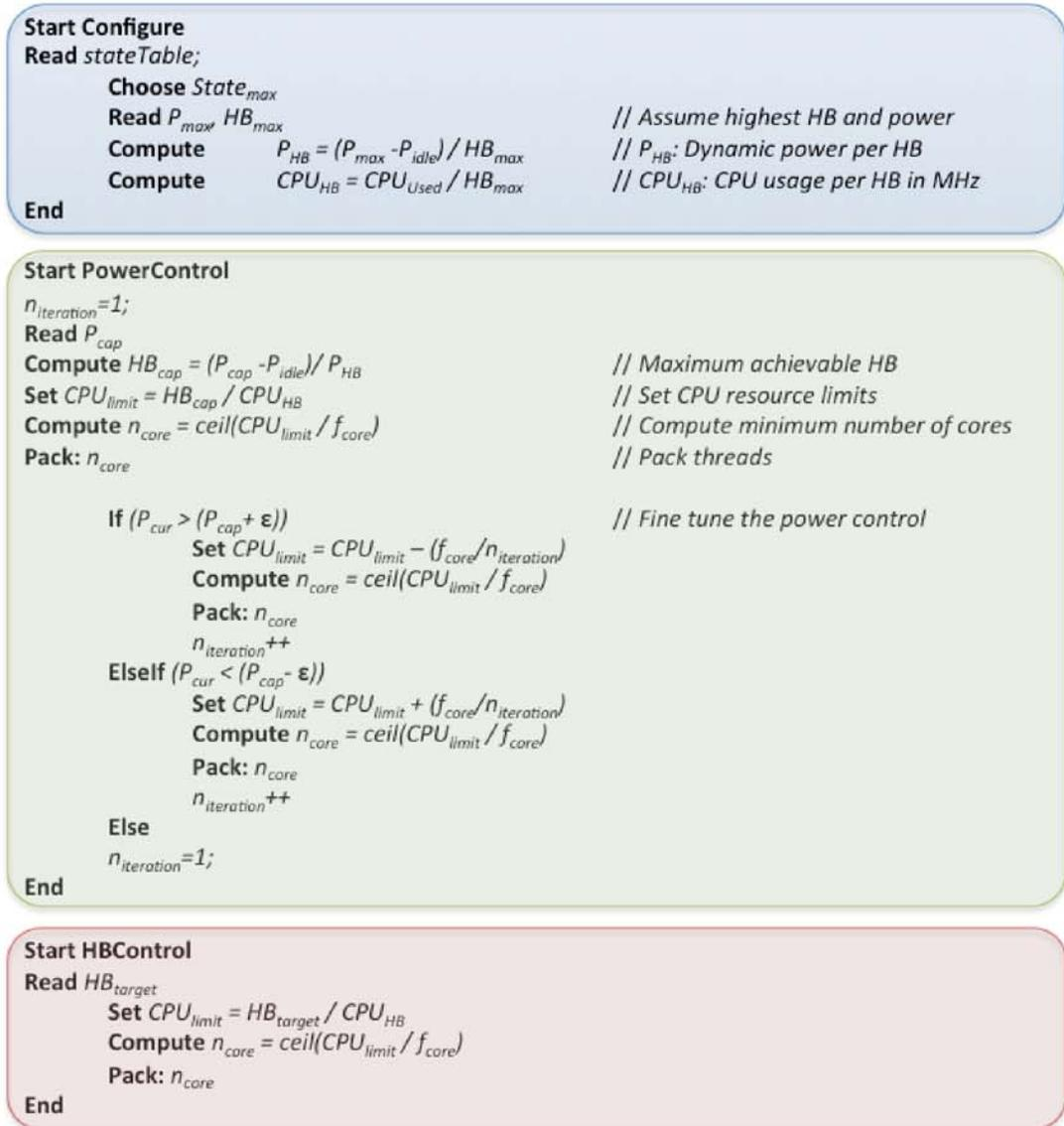
**Figure 5-20:** Pseudo-code for Adapt & Cap control modules. Adapt & Cap first discovers the higher performance application state (blue box), then periodically checks power (green box) and performance (red box) requirements to adjust its decisions.
