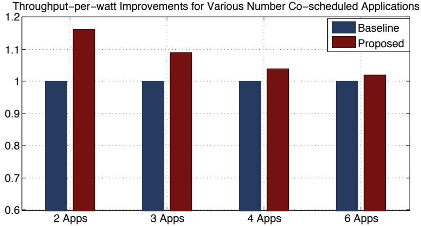
**Figure 4-20:** Normalized throughput-per-watt with respect to the baseline case, where each VM is given the maximum resources, for varying number of co-scheduled applications. Energy efficiency improvements decrease with increasing number of applications.
