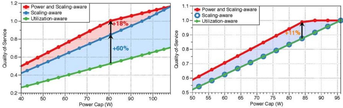
**Figure 5-11:** Total QoS comparison for consolidating two application pairs, `canneal-facesim` (a) and `blackscholes-swaptions` (b) on AMD Opteron 6172 with various power caps for utilization-based approach (baseline), naive approach (only scaling-aware) and power-aware (scaling and power-aware) approach. Power-awareness brings up to 18% and 11% QoS improvements over the scaling-only approach.
