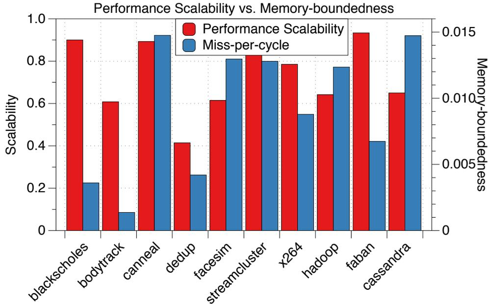
**Figure 5:4:** Memory-boundedness (last level cache misses per cycle) vs. scalability of PARSEC and CloudSuite applications. Scalability is measured as the ability to utilize the 12-core system when running with 12 threads. This experiment shows that memory-boundedness does not capture the scalability characteristics of the applications.
