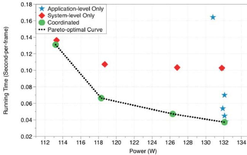
**Figure 5-18:** Power and performance tradeoff space for various adaptive techniques on Intel Xeon E5 multicore server when running x264. Proposed coordinated management extends the Pareto-optimal curve to a more efficient operating point.
