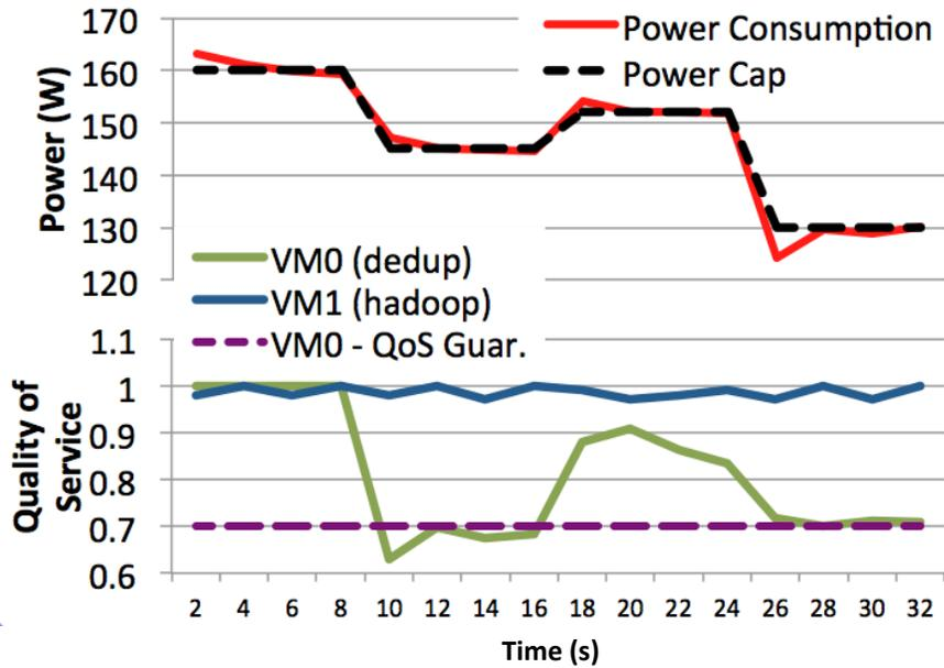
**Figure 5-9:** Runtime behavior of *vCap* under power caps and QoS constraints for the VM group running *dedup* and *hadoop*. *vCap* adheres to the power cap and ensures that the QoS guarantees are met.
