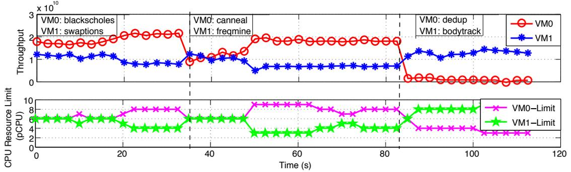
**Figure 4-16:** Runtime behavior of the resource allocation routine for 3 applications pairs. CPU resources are adjusted according to power efficiency classes of the applications to improve the overall efficiency of the server.
