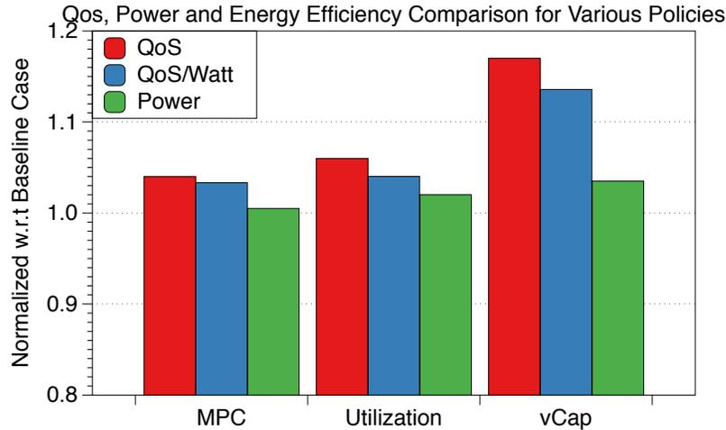
**Figure 5-8:** Comparison of QoS, QoS/watt and power consumption of the server with various consolidation techniques. The proposed technique improves the overall QoS by 17% when compared to the baseline case, where VMs have no CPU resource limitations.
