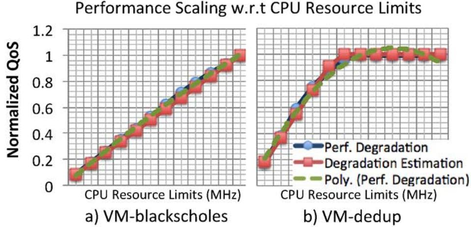
**Figure 5-7:** QoS as a function of CPU resource limits for blackscholes and dedup. Degradation estimations are derived by using Equation 5.1. Equation 5.1 provides better QoS prediction without requiring any offline/training phase when compared to polynomial models.
