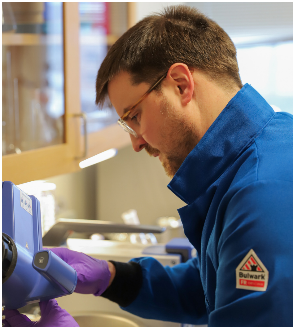
Assistant Professor Tim O’Shea showing off the rotary evaporator, used to volatilize and collect organic solvents from chemical reactions during work-up
