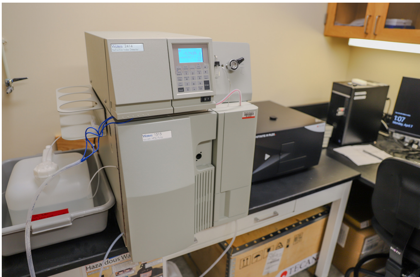
The Gel permeation chromatography (GPC) unit, used to measure the molecular weight of new polymers the O'Shea Lab synthesizes
