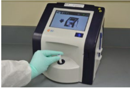
Prototype SERS reader and disposable tube containing reagents for differential diagnosis (Courtesy of Becton, Dickinson and Co.)
