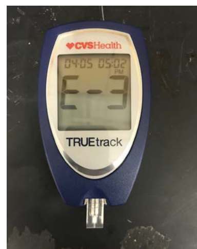
Glucometer reading wax printed test strip with silver electrode applied
