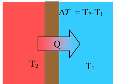
Where  $Q$  is the flow of heat energy (flow means amount per unit time, i.e., Joules of energy per second, or BTU of energy per second),  $\Delta T$  is the temperature difference across a boundary of some material,  $A$  is the surface area of the boundary and  $R$  is a measurement of how well the material hinders the flow of heat.
