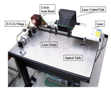
The experimental apparatus is comprised of a pulsed Nd:YAG laser (emitting at 355nm) directed through a 2-axis Scan Head. Since the pulsed UV laser is not easily visible, an auxiliary red alignment laser was used for multilevel alignment. Since light rays can be converged to a focal point, the distribution of laser intensity as a function of focal depth can be selectively exposed by varying laser doses from Gaussian-like spot.
