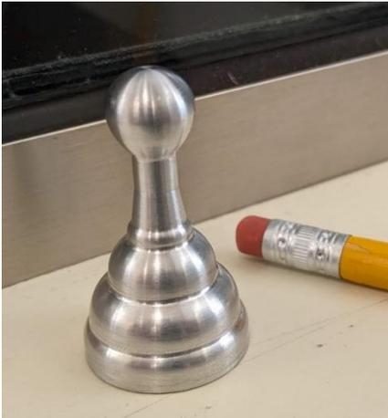
In this section you will run a PROGRAM that will machine a chess pawn using the WORKHOLDING and PART ZERO setups from the previous sections. You will be introduced to the TRAK conversational programming interface, along with the “TRAKING” feature, which allows manual control of a CNC program’s federate using the handwheels.
