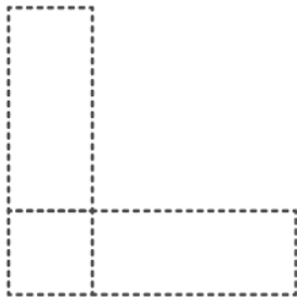
Wood Joint Half-Lap, Corner
