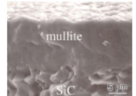
A scanning electron microscope image of a 10-micron-thick environmental barrier coating on silicon carbide.
