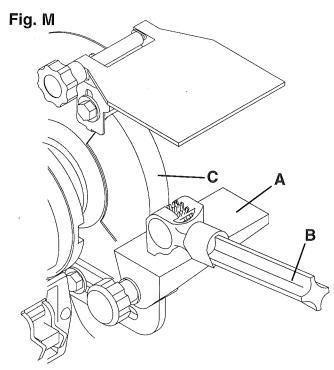
The Wheel Dresser is to be used on the grinding wheels. It will remove buildup of material on the grinding wheel, remove imperfections and make the corners of the grinding wheel square. See Figure M.
