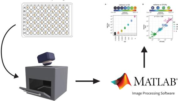
Prototyped Bioluminesense Imaging Device
