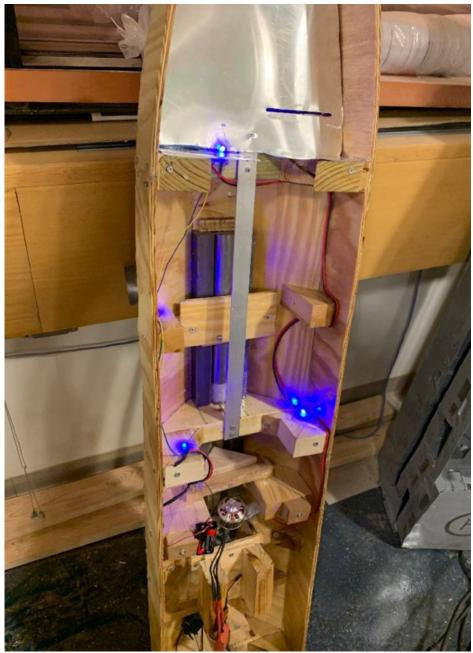
I began adding the deck for the first belowdeck level (second belowdeck level is the bilge where t he ballast and sewage tanks are). I also began adding lighting. These are blue LEDs soldered in parallel and connected to two AAA batteries and a switch with a resistor.
