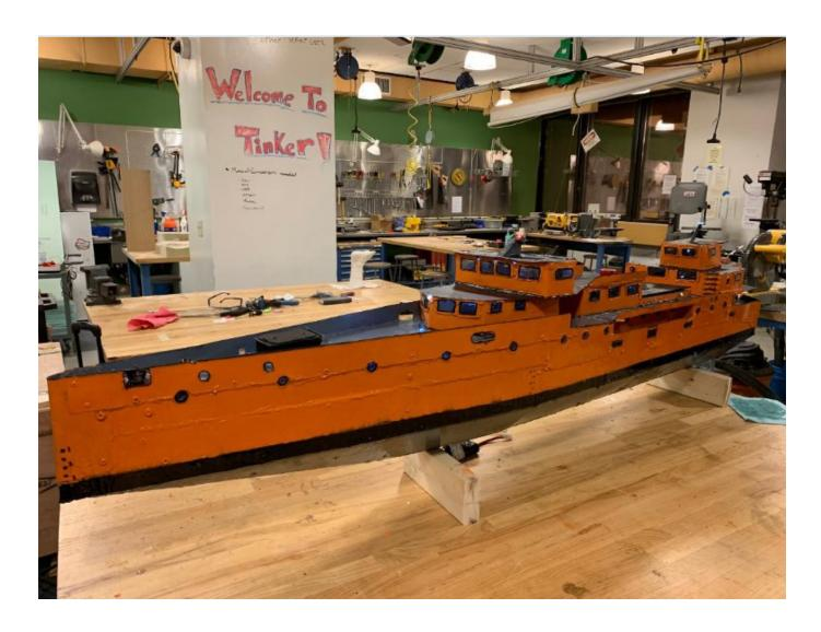
I finished painting the ship, then ensured that all cracks were caulked or hot glued. Then the entire ship was coated with epoxy to eliminate any remaining cracks.
