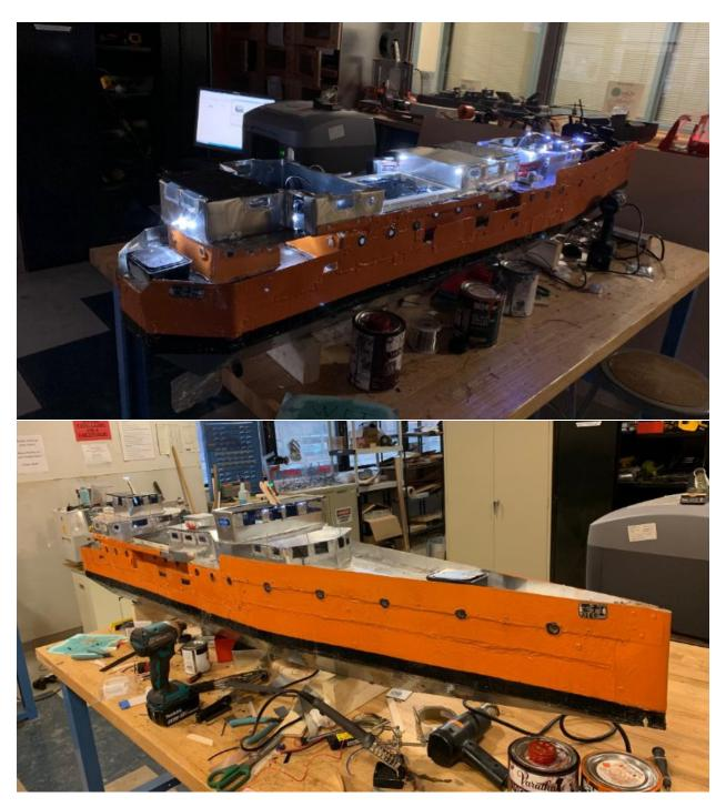
I continued building the superstructure and installing lights. There are two new lighting circuits. One powers most of the main deck lights as well as some of the crew quarters and the upper forward decks. The other illuminates the rest of the upper decks and powers the navigation lights. Note that the nav lights are backwards in this picture due to distracted gluing. This was subsequently fixed.
