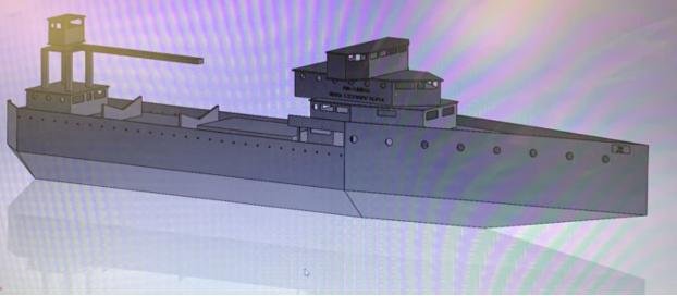
At this point, I measured what I had built so far and created a Solidworks model of it. I also added a preliminary superstructure design.
