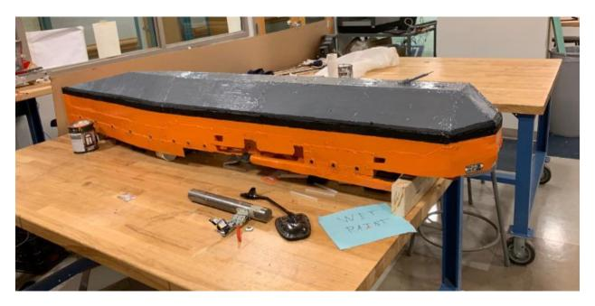
At this point, the ship was turned upside down and the outer hull was coated with epoxy. Once the epoxy cured, the hull was painted, then coated with more epoxy. I also made name plates.
