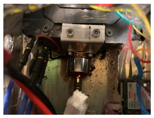
After recovering *Zureteiku*, I assessed the motor mount design and decided to reconfigure it. As the motor had been installed before the superstructure, the screws holding the motor mount to the bulkhead were now nearly impossible to reach. Therefore, I designed the L-shaped aluminum bracket in the above figure to hold the motor. To replace or maintain the motor, the bracket (with motor attached) can be removed by unscrewing the two easily-accessible top screws.
