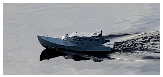
Initial sea trials revealed that the hull was responsive to rudder input during maneuverability tests, as well as relatively efficient, judging from the relatively small bow wave, and also by the lack of churning foam at the bow. This testing was conducted with a 7.4 V (2S) LiPo battery.
