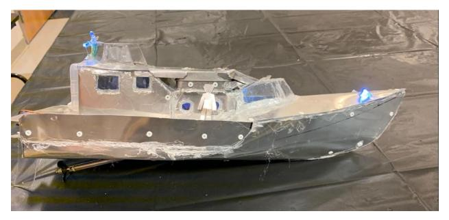
As seen above, the rest of the hull was built from the same aluminum flashing. LED lights are connected to the radio receiver, which regulates the voltage that they receive. Usually, this is sufficient, but in this case, the lights shown here burned out in approximately a week, and needed to be replaced with new lights, this time with a resistor in series. The cut-out figure is used to determine appropriate feature scaling; this figure represents a 6' tall person in 1/32 scale.
