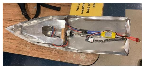
The hull is built with aluminum flashing. This is a thin metal, usually bought in large rolls, which is manipulable by hand, but thick enough to be used structurally if designed appropriately. After temporarily duct-taping the seams, hot glue (for sealing) is added, and then the seams are blind-riveted together. In this photo, it can be seen that the motor is directly attached to the wooden bulkhead; this caused problems that are described in more detail below.
