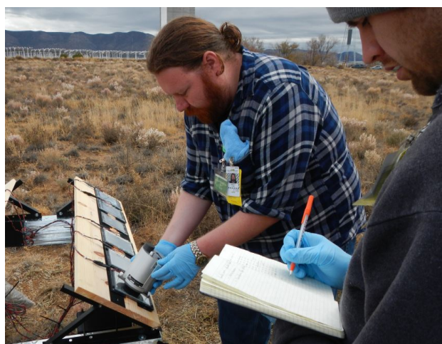
Stark (left) and Hudelson taking a specular reflection reading last year on mirrors they installed at Sandia National Laboratories in Albuquerque, N.M. Photo courtesy of Jeremy Stark
