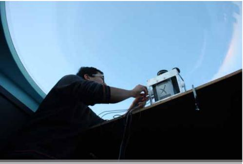
Ph.D. student, Hassan Akbari (ECE), installs a low-light imaging system in an observing dome at the Poker Flat Research Range near Fairbanks, Alaska. The camera system is used to study fine-scale structure in the aurora borealis and its relationship with plasma turbulence in the ionosphere.
