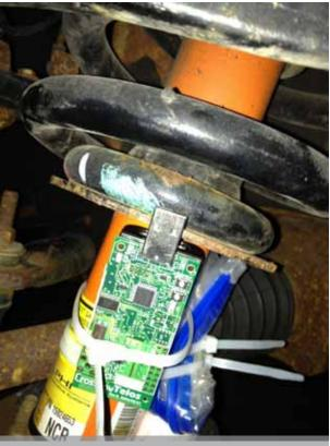
The research team tested out sensors, like this one attached to the suspension system of the front wheel, on a Cadillac Escalade.
