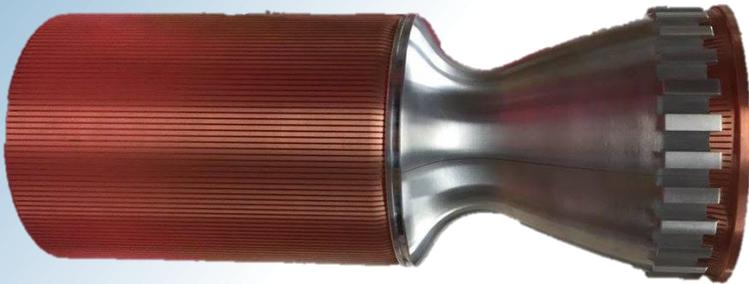
*Copper chamber and aluminum saddle after machining. Regen channels clearly visible*
