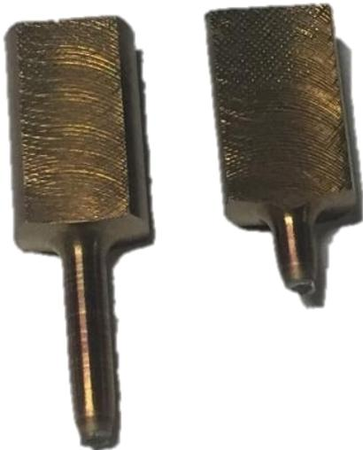
*Heat treated steel after tensile testing*
