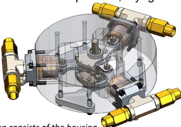
Pump consists of the housing, pistons, and center linkage. The piston manifolds have check valves on their inlets and outlets to determine flow direction
