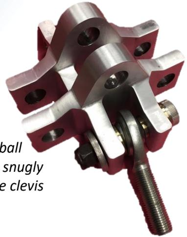
Rod end ball joint fits snugly on engine clevis
