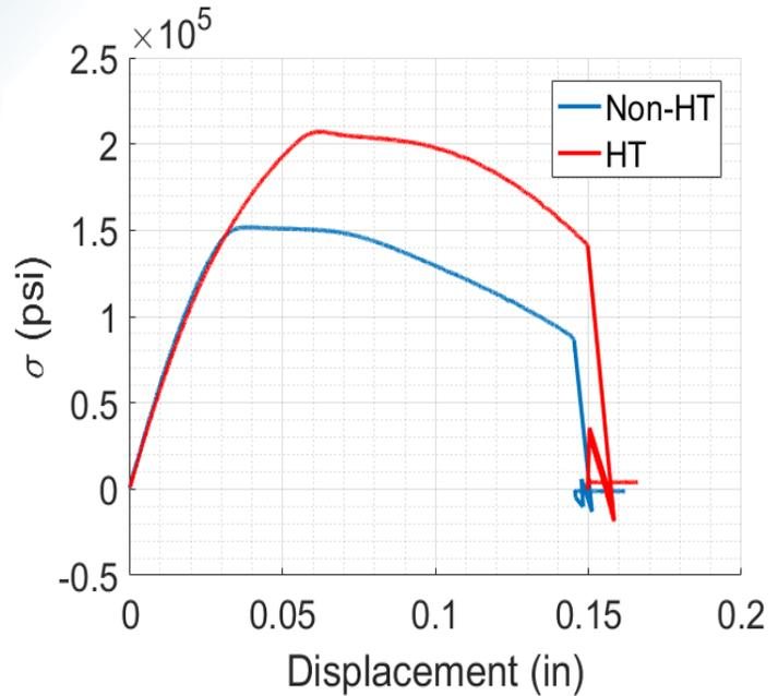
*Tensile testing results for heat treated and non-heat treated steel samples*
