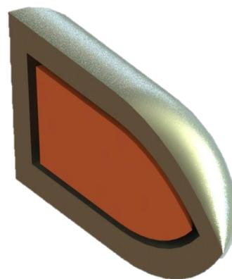
Simplified RTG CAD model: Tungsten shell with red-hot plutonium inside
