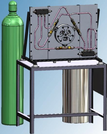
Full CAD assembly of pump, test stand, pressurant bottle, water tank, and motor (behind panel)
