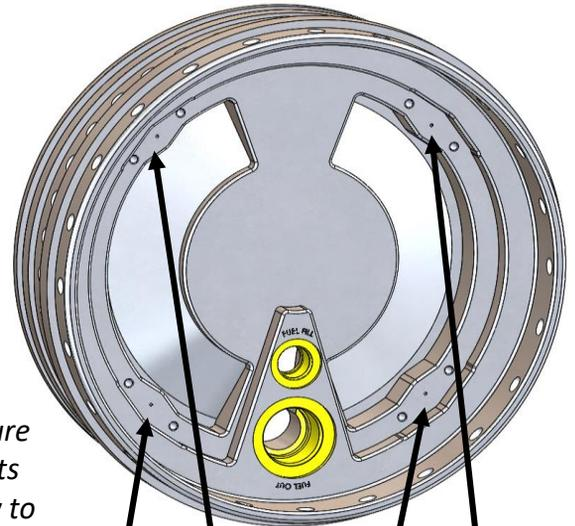
Structure mounts directly to location-defining features on the aft fuel bulkhead
