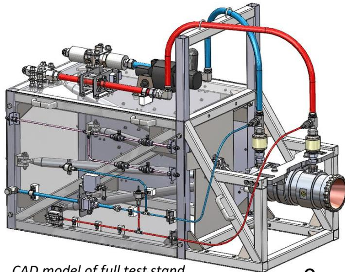
CAD model of full test stand showing internal thrust structure
