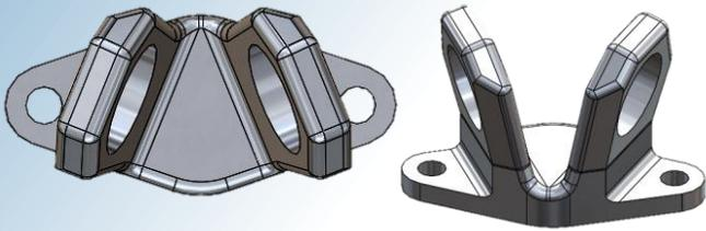
The 8 load transfer units (4 on bulkhead, 4 on engine mount) will have 3/16" spherical joints press fit in to avoid static indeterminacy
