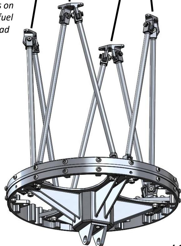
Thrust structure CAD model
