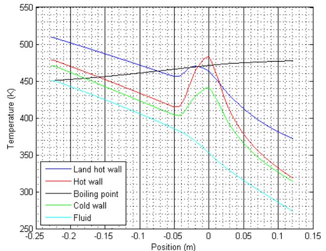
*Steady-state temperatures vs axial position*
