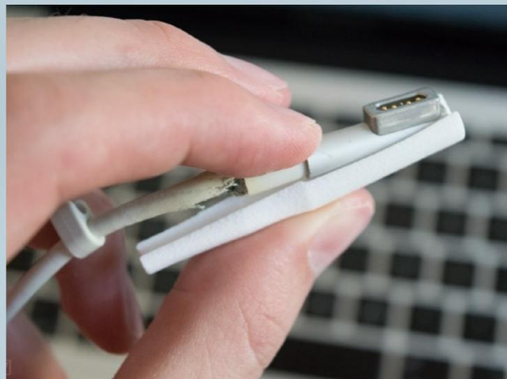
With this, one can press the metal end of the connector into the case, and then press the cord and its potentially frayed parts into the lower portion.
