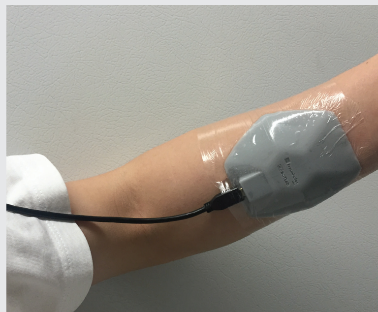
Before testing the wearable sensors on patients, Roblyer tests early designs of his devices on the wrists of healthy volunteers to see how well it measures blood flow and water and fat content. Photo courtesy of Darren Roblyer
