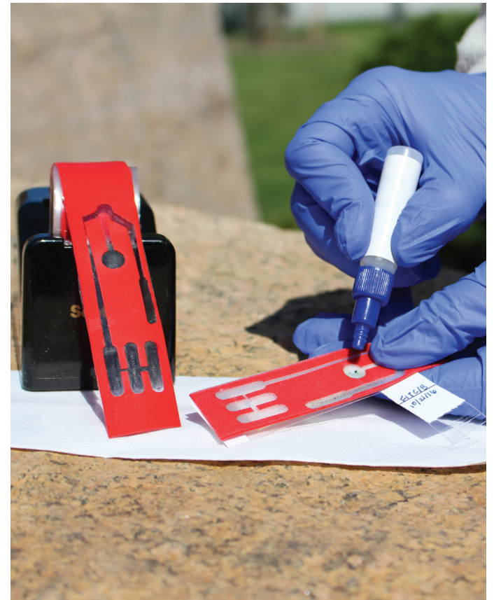
SNAPflex (System for Nucleic Acid Prep-Flexible) can be used in low-resource areas to extract, prep, store and ship patient samples as a low-cost and simple method to consistently monitor HIV-infected and high-risk patients.
