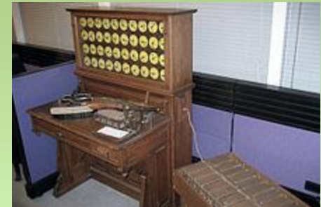
Hollerith tabulating machine and sorter
