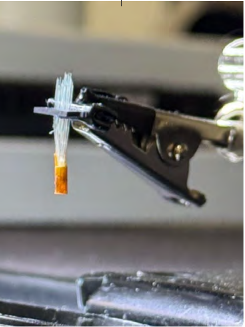
This fiber array is used to record optical measurements of neural activity in the brain of a mouse, allowing scientists to study the neural circuits.
