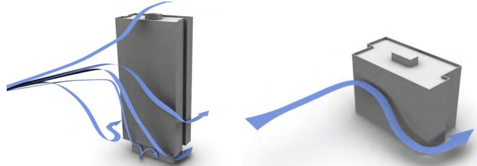
**Image 5a – Downwashing Flow (Left) Corner Acceleration (Right)**
