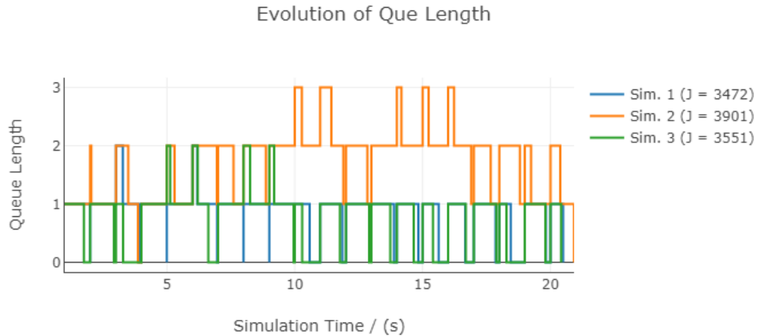
Figure 9: Case 2: Arrival times are deterministic, required quality levels are uniformly distributed, all penalty parameters are equal to 1, and Sim.1 - Sim.3 respectively stands for when the control input is generated via a) Forward algorithm, b) Deterministic with u_i = 3, \forall i and c) Uniformly distributed where u_i \sim U[3, 5]
