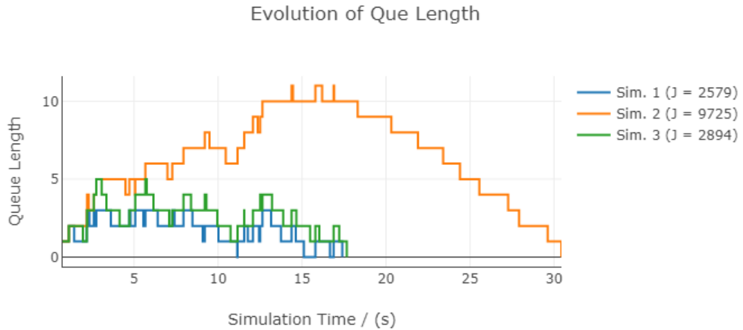
Figure 7: Case 1: Arrival times are Poisson distributed, required quality levels are uniformly distributed, all penalty parameters are equal to 1, and Sim.1 - Sim.3 respectively stands for when the control input is generated via a) Forward algorithm, b) Deterministic with u_i = 2, \forall i and c) Uniformly distributed where u_i \sim U[2, 5]
