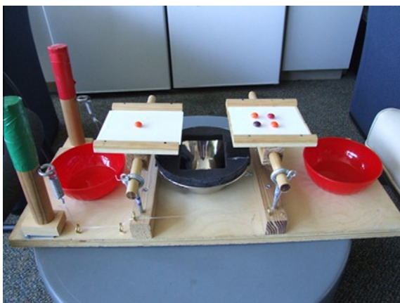
Fig. 1. Apparatus. Children sat face-to-face with one, the decider, controlling the two handles. Pulling the green handle caused the trays to tip outward, dropping the candies into the bowls for each player. Pulling the red handle caused the trays to tip inward, dropping the candies into the center bowl for rejections. (For interpretation of the references to color in this figure legend, the reader is referred to the web version of this article.)
