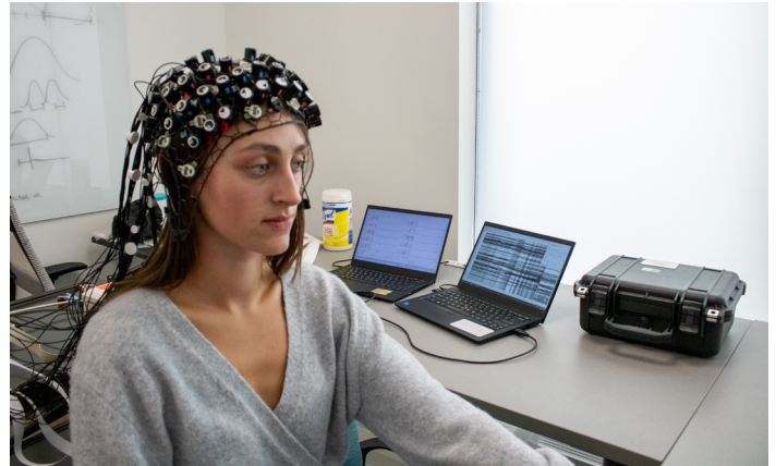
Helen Blans wears the fNIRS-EEG equipment to demonstrate how the data collection process works.
