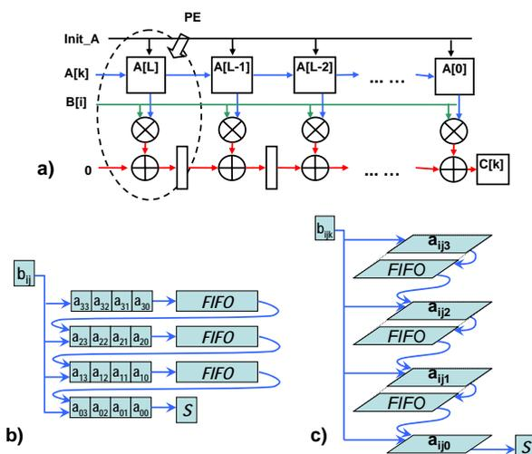
Figure 5: Shown are a) a one dimensional systolic convolver array, and its extension to b) two, and to c) three dimensions.
