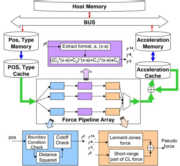
Figure 2: Pipeline for short-range force computation.
