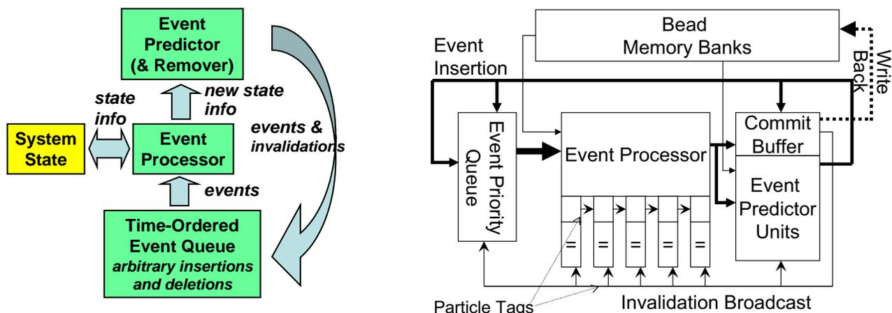
Figure 6: Shown are block diagrams of a) a generic Discrete Event Simulation and b) an FPGA mapping of Discrete Molecular Dynamics.
