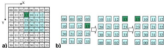
Figure 4: Shown is an example of a 2D interleaved memory reference. a) Shows the grid points (shaded) to be recovered. b) Shows the two rotations needed to get the shaded points into correct position.
