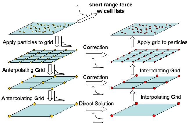
Figure 3: Schematic of the multigrid method for the Coulomb force.
