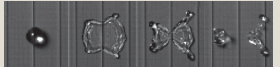
A droplet that lands on a surface with added ridges—about the size of a human hair—bounces off in 7.8 milliseconds.
