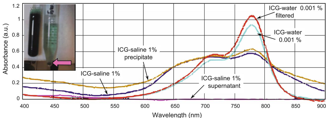
**Fig. 1** ICG absorption spectrum: *Inset* ICG is freely soluble in water but not in saline in which it precipitates (*pink arrow*). In water, ICG produces a characteristic spectrum with peak absorbance at 780 nm
