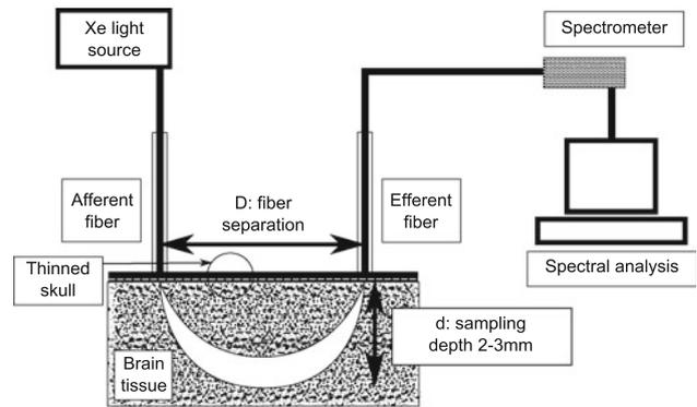
**Fig. 2** Set-up for the optical pharmacokinetic device that uses a variation of diffuse reflectance spectroscopy for measuring concentrations of absorbers in turbid media
