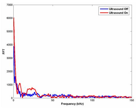
Fig. 4. FFT of one peak obtained with the ultrasound off and one peak obtained with the ultrasound on.
