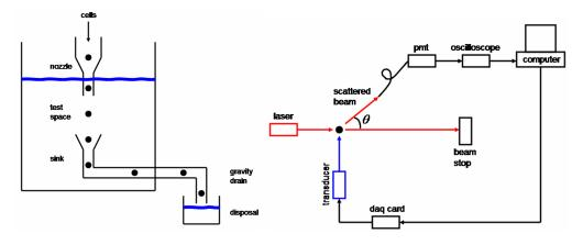
Fig. 1. Laminar flow setup.
