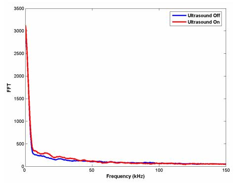
Fig. 5. Averaged FFTs of 75 peaks obtained with the ultrasound off and 75 peaks obtained with the ultrasound on.
