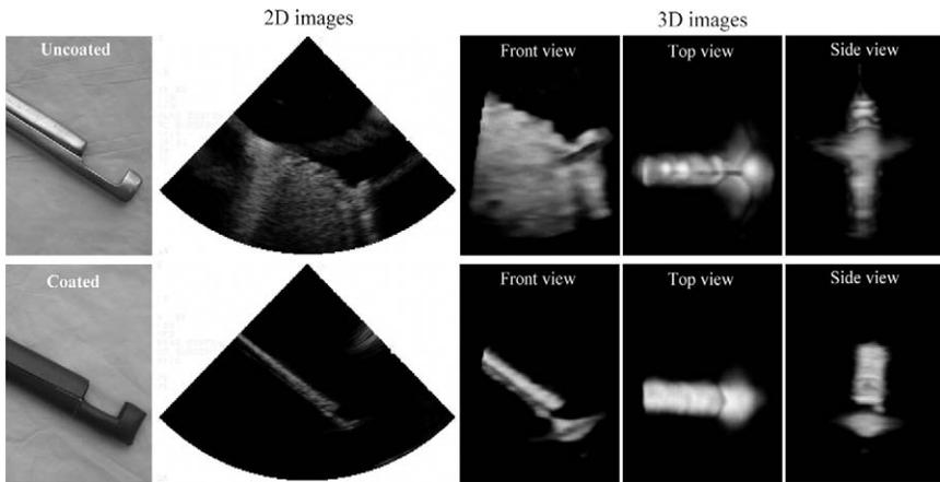
**FIG 10.** Effect of polyurethane foam coating on suturing device imaging. (Top row) Uncoated. (Bottom row) Coated with polyurethane foam. (Reprinted with permission from Huang et al,<sup>31</sup> ©2007 American Institute of Ultrasound in Medicine.)
