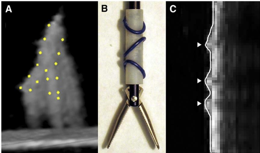
**FIG 3.** Ultrasound imaging of forceps. (A) Three-dimensional image of forceps with actual location indicated by dots. (B) Fiducial marker on shaft of forceps. (C) Ultrasound image showing detected locations of marker ridges (arrowheads). (Color version of figure is available online.)
