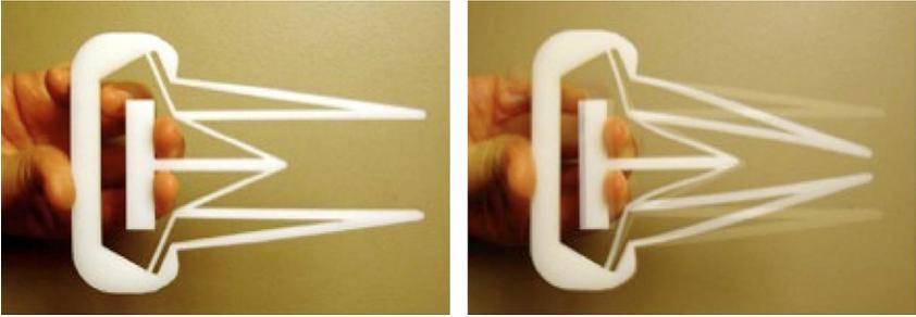
**FIG 9.** Prototype of the compliant gripper in its inactive mode (left) and gripping mode (right). (Reprinted with permission from Kota et al.<sup>46</sup>) (Color version of figure is available online.)
