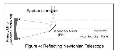
The first telescope design that used mirrors instead of lenses was invented by Isaac 1680. Newton in The objective in this design (see Figure 4) is a concave parabolic mirror, which reflects light onto a flat secondary mirror, moving the focus of the primary outside of the path of the light rays entering
