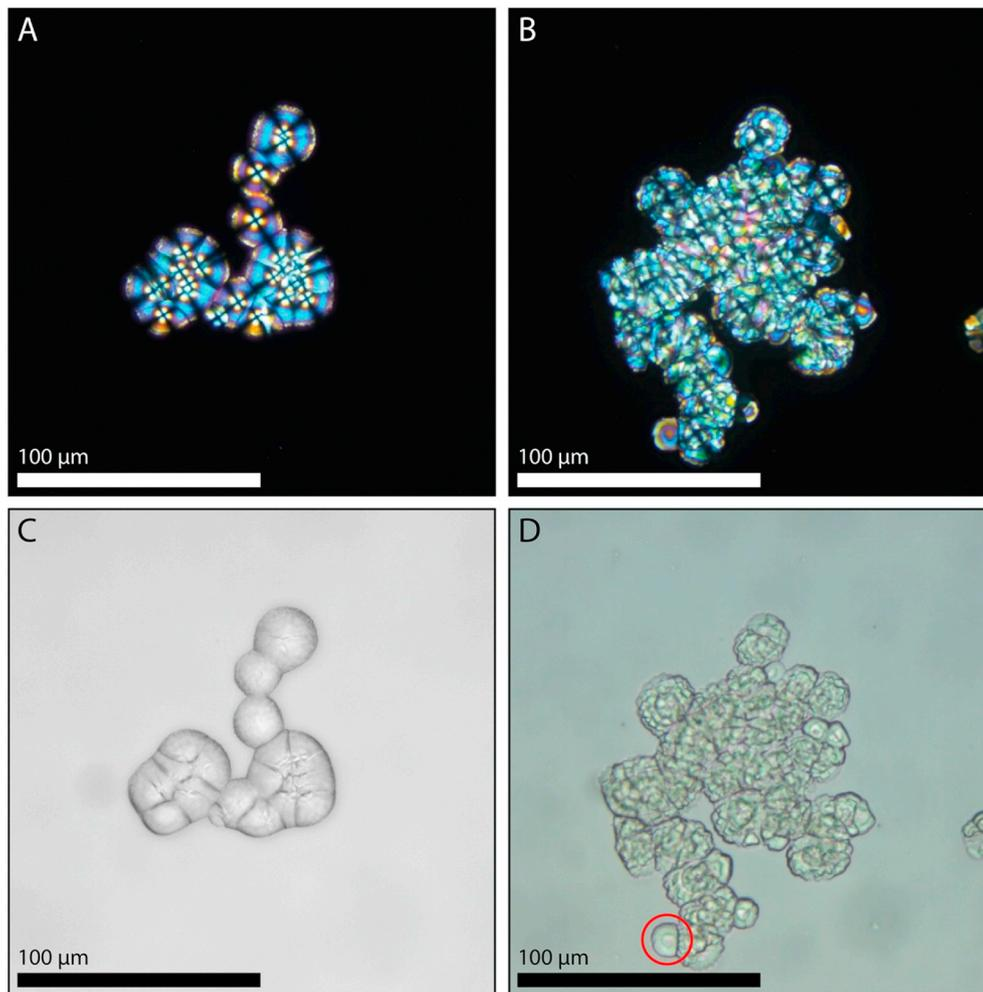
**Fig. 3.** Maize starch structures skimmed from the surface of an alkaline solution after 48 h (A, C) and 120 h (B, D) of soaking with no heat (Trial 4). Highlighted particle is smoother and appears “newer” than other particles visible in D.
