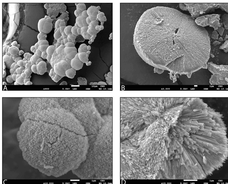
**Fig. 5.** Nixtamalized starch particles observed under scanning electron microscopy. Entire structures (A), and their surface texture (C), are revealed as radial bundles of linear crystalline structures at higher magnifications (D) and when particles are broken open (B).
