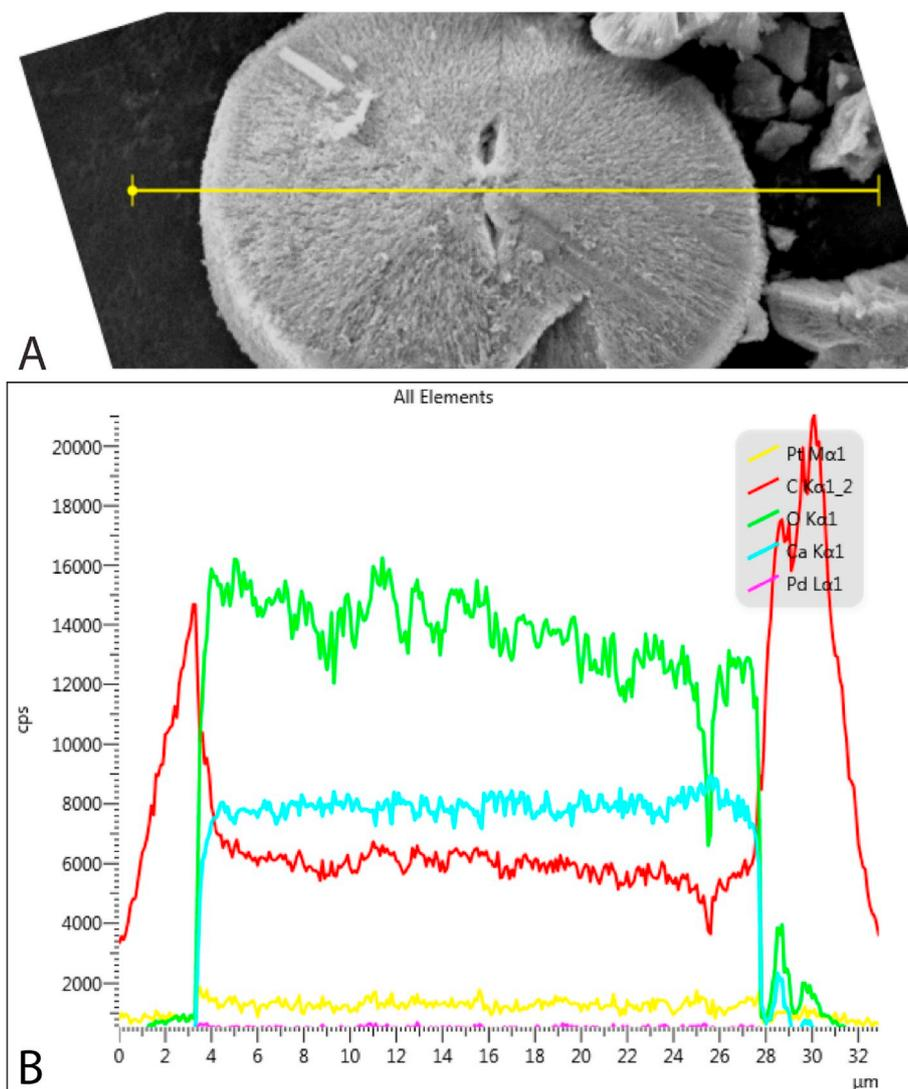
**Fig. 6.** SEM-EDS image (A) and spectrum (B) of nixtamalized starch particle shown in Fig. 5B. Pt and Pd are present due to sample coating; carbon readings below 4  $\mu\text{m}$  and beyond 28  $\mu\text{m}$  are measurements of the carbon tape on the stub. Hydrogen cannot be detected by this instrument.
