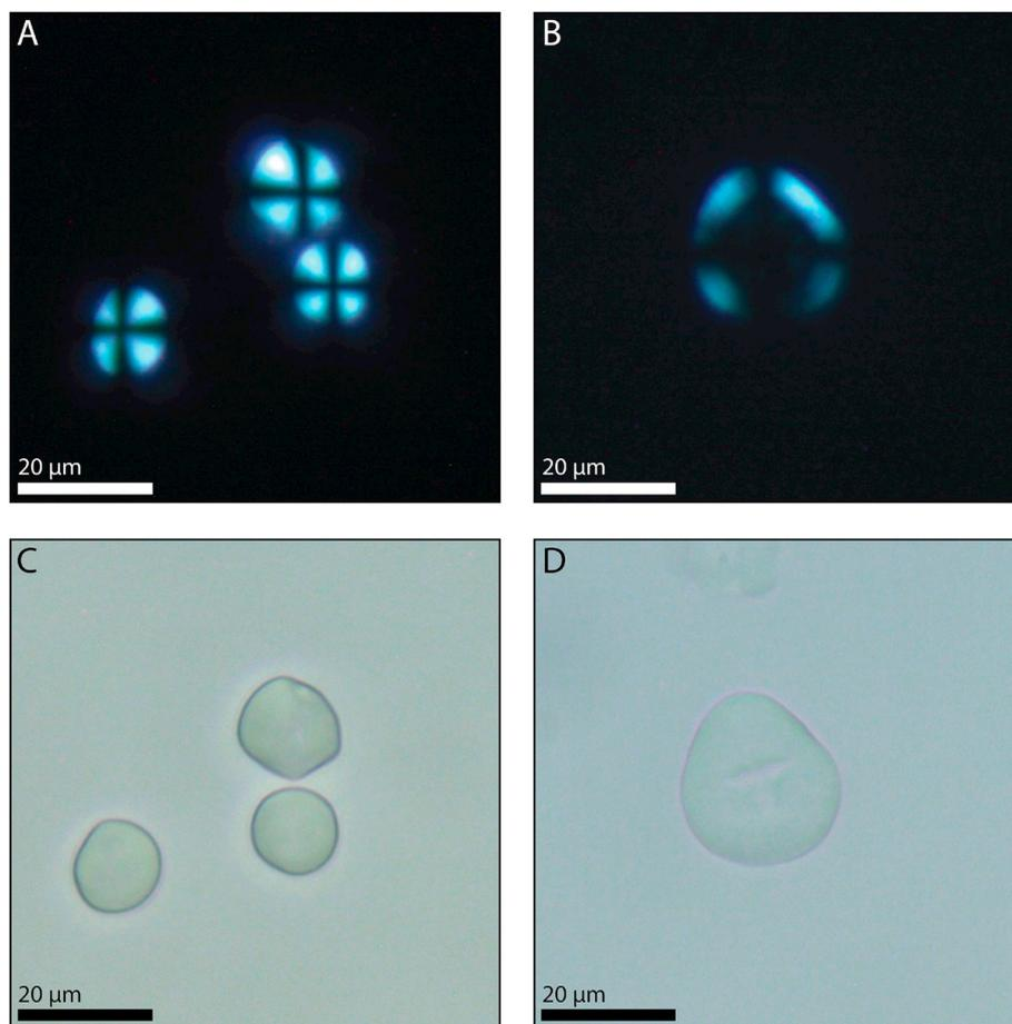
**Fig. 1.** Images A and C (Trial 2, 0 h) display unaltered maize starch morphologies in cross-polarized and brightfield light, respectively. Images B (cross-polarized) and D (brightfield) show a boiled starch granule displaying a typical “boiled” morphology including swelling, a loss of birefringence, and expansion of the hilum (Trial 8, 100 min).
