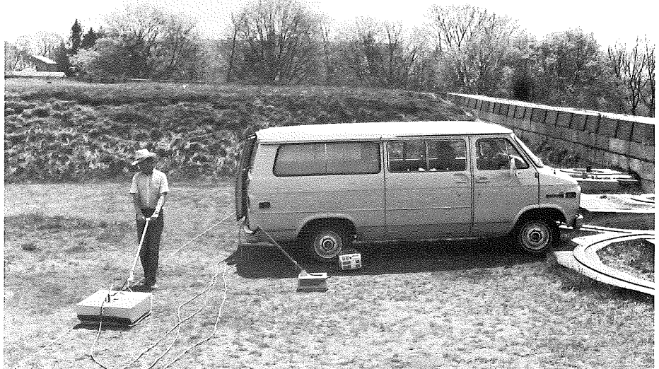
Dr. Bruce Bevan, of Geosight, Inc., conducting a survey using ground-penetrating radar at the river battery.
